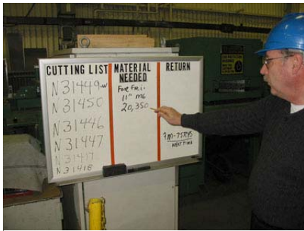
The above communication Whiteboard supports a Kanban system for replenishing steel coils and sub assemblies in the stacking area.
