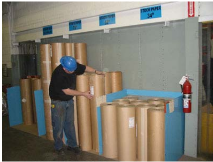
5S organization of the duct paper storage area freed up 50% of available floor space.
